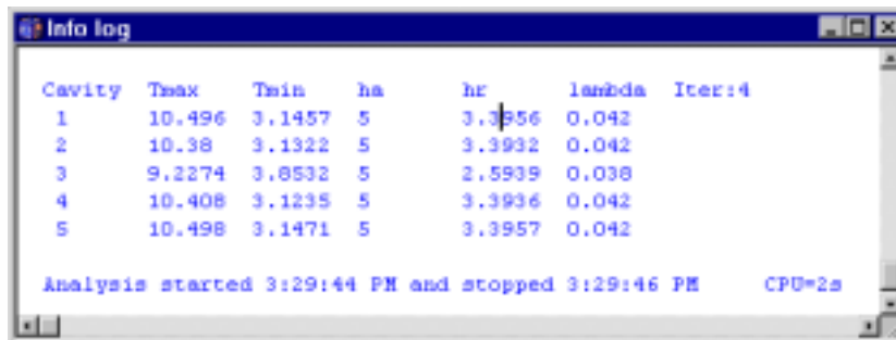
Figure 10.8: The info log shows here iteratively calculated temperatures when option 4 is used. The text indicates that four updates have been made for calculating the equivalent thermal conductivities. Compare equivalent thermal conductivities with those in the above figure.
