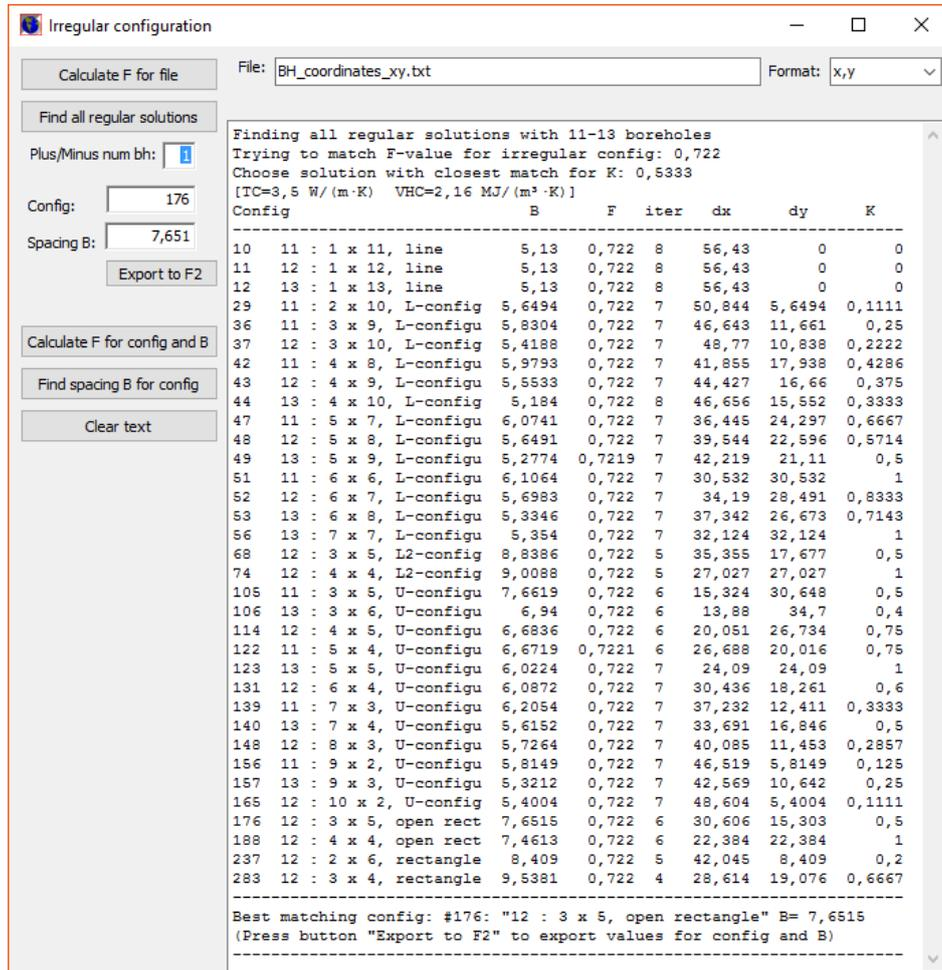
“Export to F2” will copy the values for configuration number and spacing B to window “Borehole and heat exchanger” (F2).
