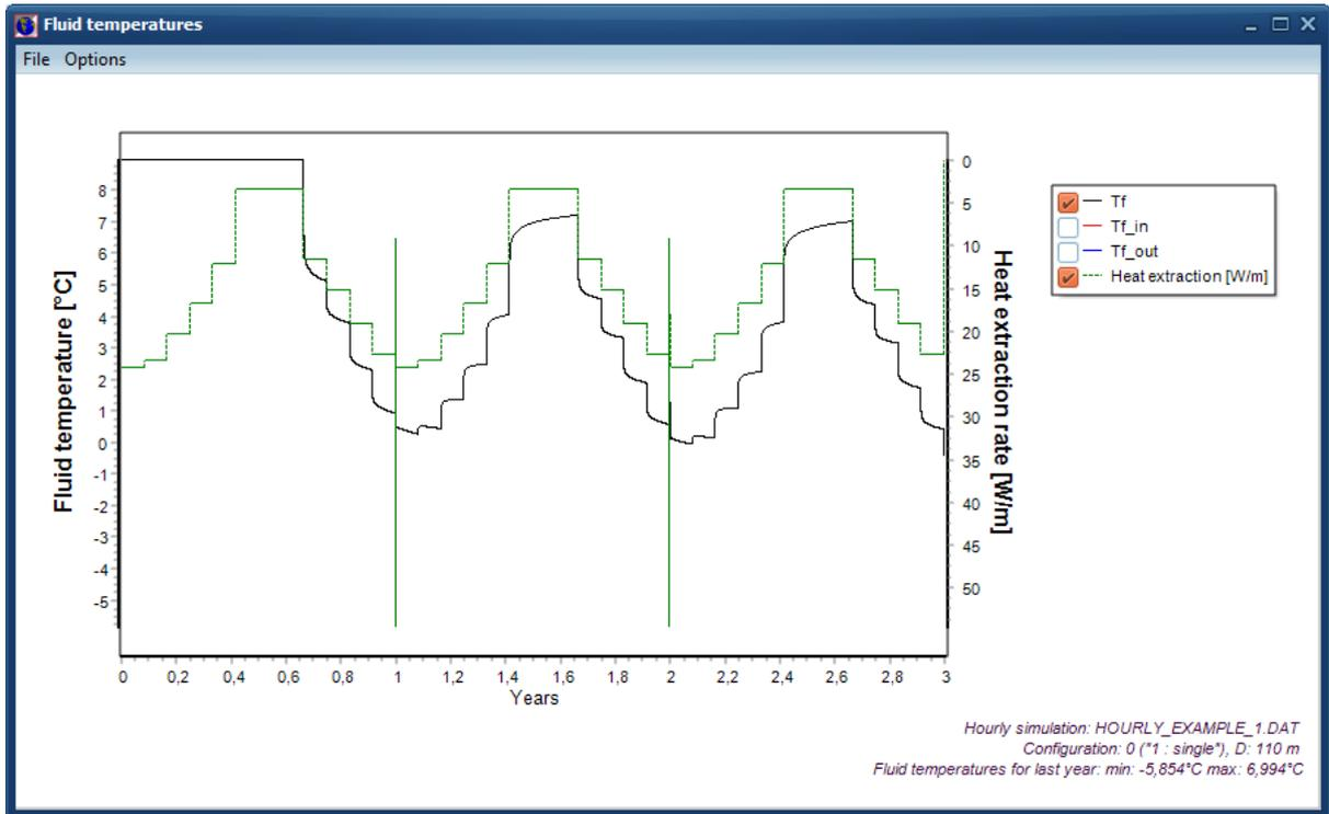
Zoom the area around  $t=1$  year (here we have first changed the time label to hours in menu item “Options”). The ground heat injection value at e.g.  $t=3h$  (and  $t=8763h$  and so on) has the value  $-6000$  W which gives  $54,54$  W/m for one borehole with depth  $110m$ .
