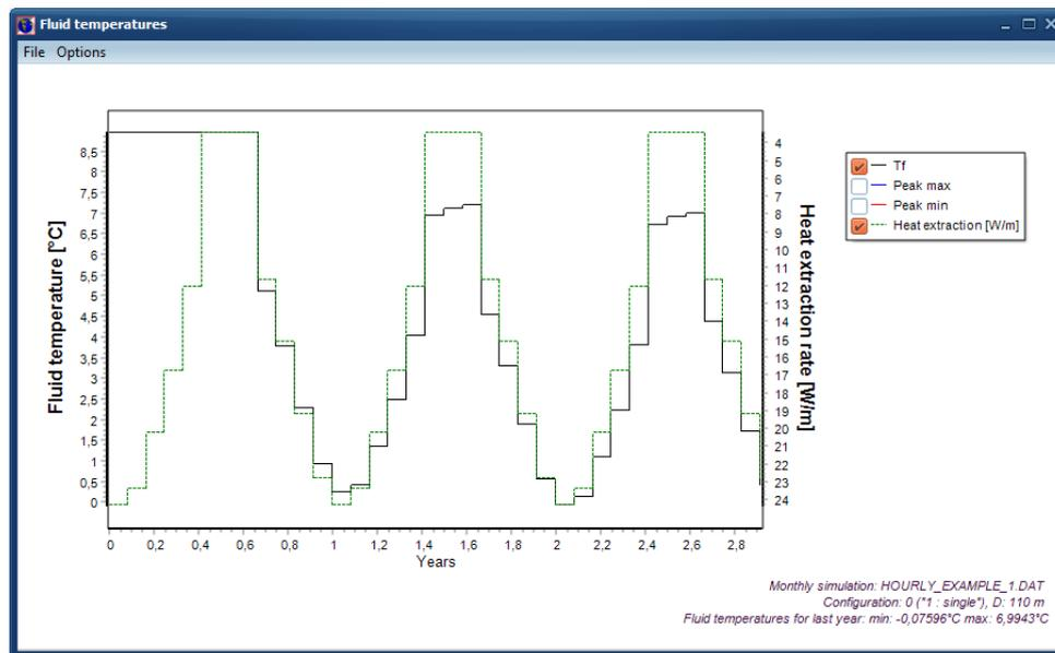
The heat extraction is  $2674/110 = 24,31$  W/m for January, just as we calculated before.
