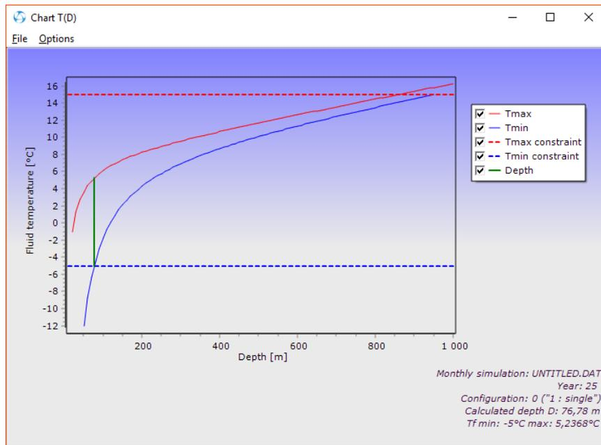
The min/max fluid temperatures are here given by:
