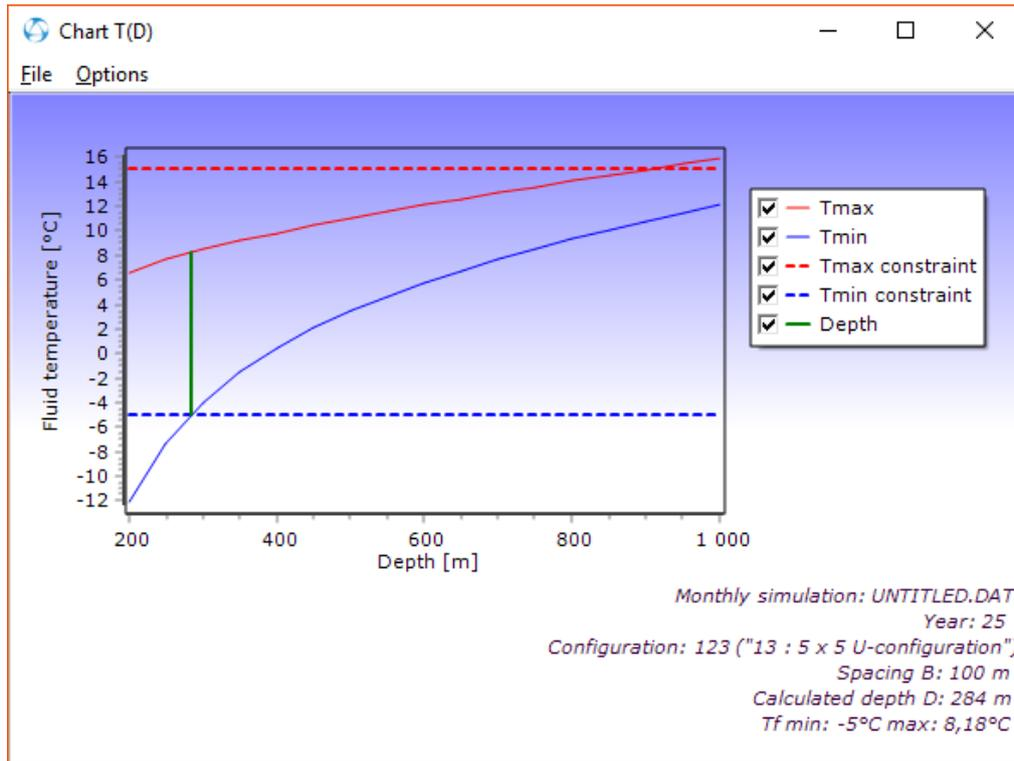
The calculated length 284 m (or more exact 283,74 m which is the same value from the optimization list) will be inserted in the menu below.
