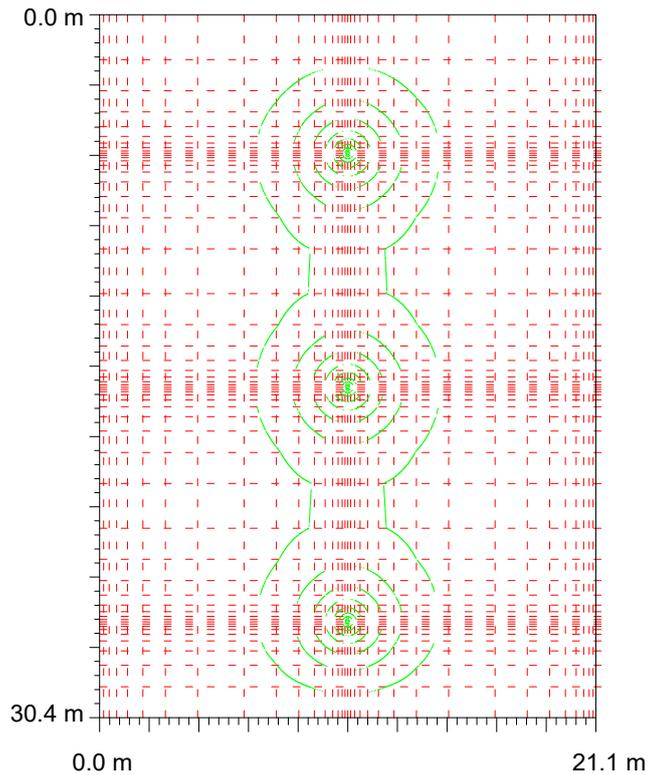
Figure 1: Temperature distribution (isotherm pattern) around 3 BHE, horizontal cross section in 50 m depth, after 8 month of winter operation (After SZAUTER 1998)
