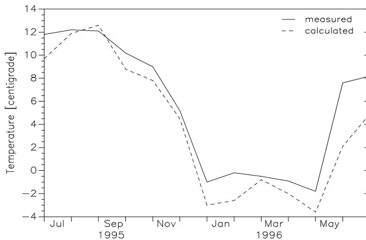
Fig. 2. Measured and calculated brine temperatures for UEG plant, Wetzlar (after HELLSTRÖM et al. 1997)
