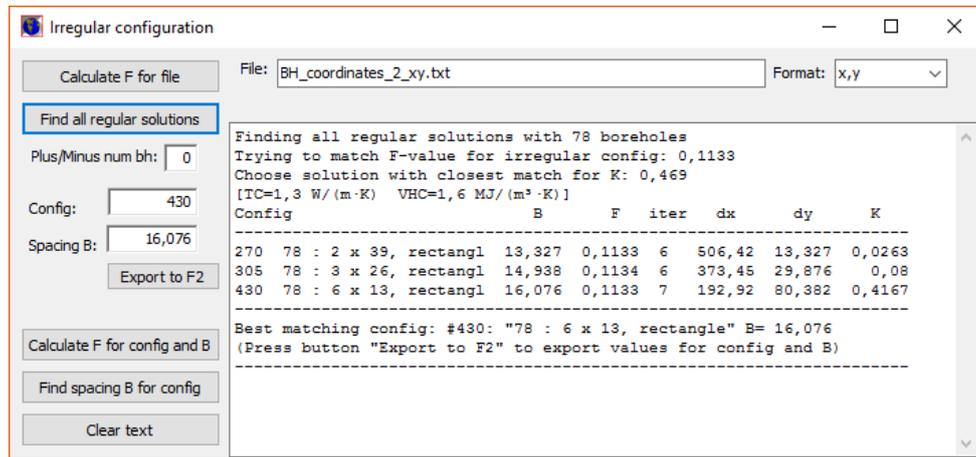
The best matching configuration 430 gives an error of about 0.4 °C compared with the results for the original configuration using SBM. This case is a bit more difficult to approximate due to that the configuration has two “groups”.
