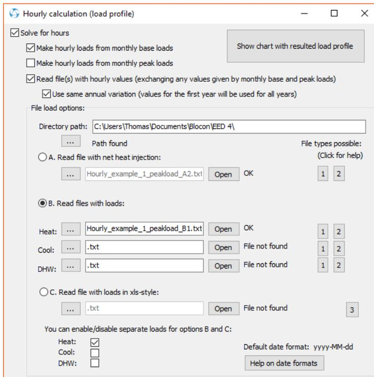
See file “Hourly\_example\_1\_peakload\_B1.txt”. In this case we have the peak load 5 kW. However, since the value in menu item “Peak load” replaces the base load value (heating + DHW) we need to subtract the DHW ( $5 \times 6/8760 = 0,5708$  kW) since it is included in the base load from “Make hourly loads from monthly base loads). (This is ok since the SPF-value is the same for the heat load and the DHW load in this case.)
