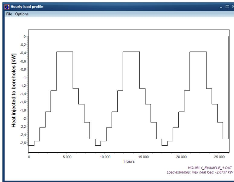
As shown above, the heat extraction from the ground is  $1,952e6/730=2674$  W during January.
