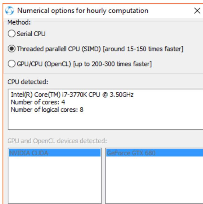
The default (and recommended) method is “**Threaded parallel CPU SIMD**” which is 15-150 times faster than “Serial CPU” (as used in previous versions EED v1.0-v4.13).
